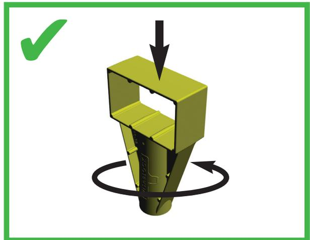
Apply the block using a twist and push down action
